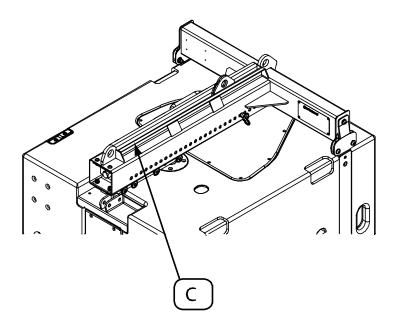
D. Two safety lifting lugs are provided for attaching wire safety rope. No other part of the flybar can be used for this purpose.
