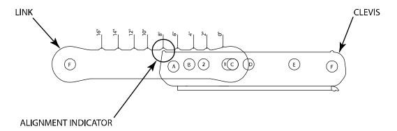
The following table shows the position of the rear link relative to the cabinet clevis to achieve the required intercabinet angle.
