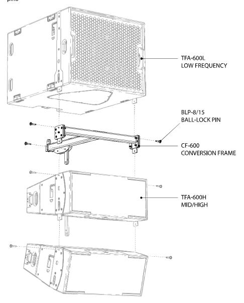
Connection to the first TFA-600H cabinet is made via two 10mm ball-lock pins which are engaged into the rear spine of the mid/high cabinet (one pin is located on the loudspeaker and one pin is located on the conversion frame).
