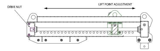
Turning the drive nut on the end of the shaft the lift point moves along the rear spine, tilting the load by varying the motor connection point relative to the centre of mass of the cluster. The screw is located in polymer sealed bearings requiring no maintenance under normal operating conditions, and is designed to last the lifetime of the product.
